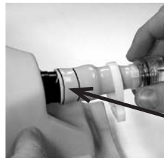
Photo 6 (Area where clamp is placed.)
